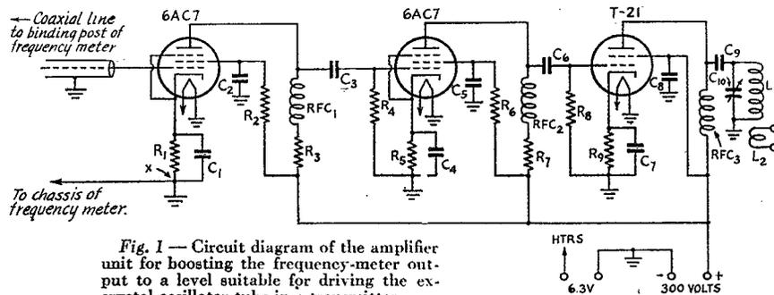
Fig. 1 — Circuit diagram of the amplifier unit for boosting the frequency-meter output to a level suitable for driving the external crystal-oscillator tube in a transmitter.
